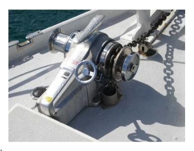
maintenance is now simply new oil in the gearbox and plenty of grease on the moving parts. For any windlass motor, I can recommend a liberal coating of CRC Soft Seal on the motor for a long life.
